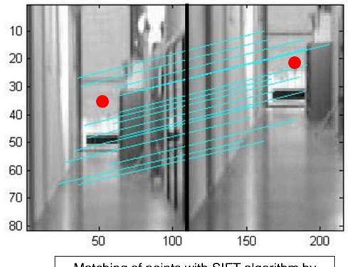
Matching of points with SIFT algorithm by D.G. Lowe, US Patent 6,711,293, filed 1999
